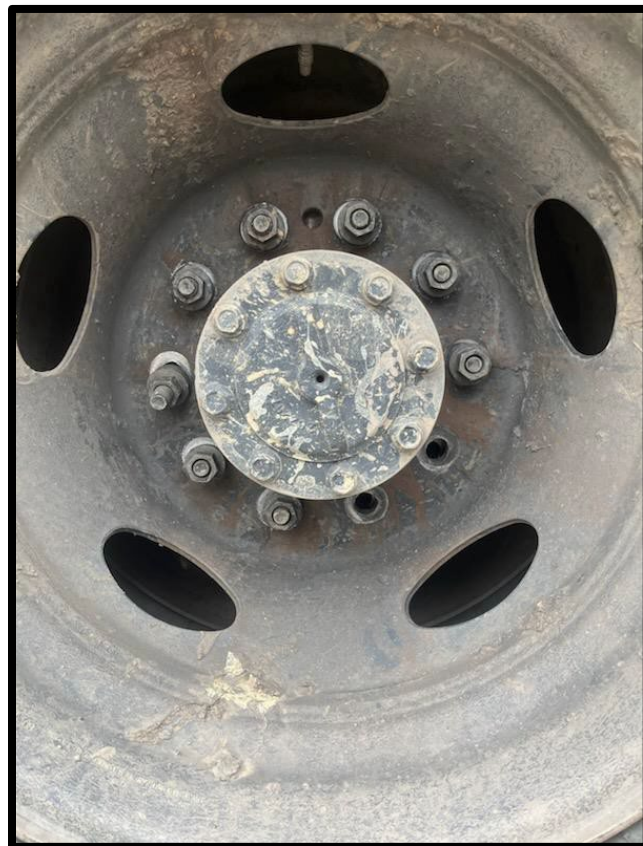
Photo 1: The wheel rim of a rear tire shows two missing lug nuts.
