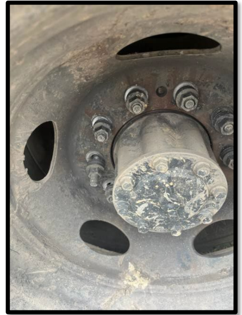
Photo 2: Note the exposed metal around the tops of the lug nuts.
